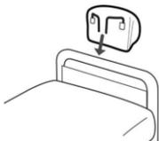
**With a cable holder:** Place the power cable in the cable holder of the mattress by opening the press studs, placing the cable in the gap and closing the press studs again.
