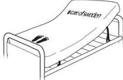
If the mattress is used on an adjustable bed, the straps shall be fastened to the non-movable parts of the bed. The straps at the head end of the bed shall be fastened at the moving part of the head end. The straps at the foot end of the bed shall be fastened at the moving part of the foot end.
