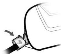
4. Check that the switch on the side is set to '0' (off). Plug the power adaptor into an easily accessible approved electrical socket (100-240 V).
