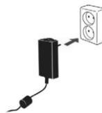
The power adaptor is part of the equipment and may not be replaced. If the control unit has been stored in its minimum or maximum storage temperature (-25°C or 70°C), wait at least 1 hour before starting it. This time is based on an ambient temperature of 20°C.
