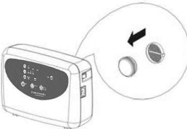
1. Loosen the small, round protective plate on the back of the pump.
