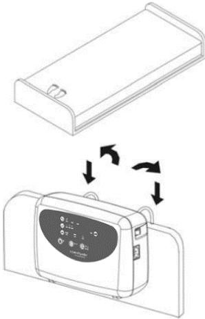
1. If the mattress has an integrated foam cushion (CuroCell® AUTO4) then the mattress is placed directly on the bed base. Secure the mattress to the moving parts of the bed using the straps on the cover.
