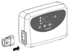
3. Connect the air tubes from the mattress to the side of the pump. A click is heard or felt when they are correctly connected.
