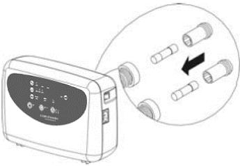
1. Remove the plug from the wall socket when replacing fuses.
