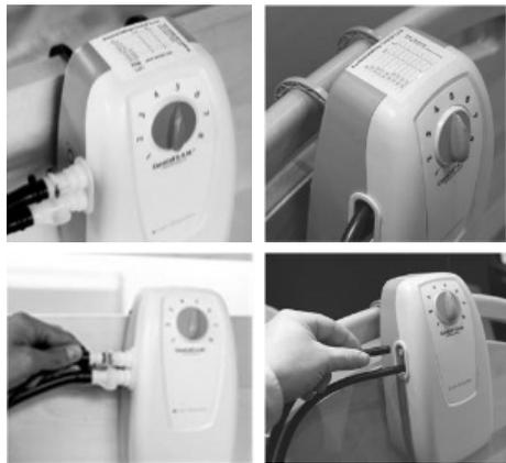
4. Check to make sure that the power is set to '0' (off). Plug in the power cord into an approved outlet (220 V).
